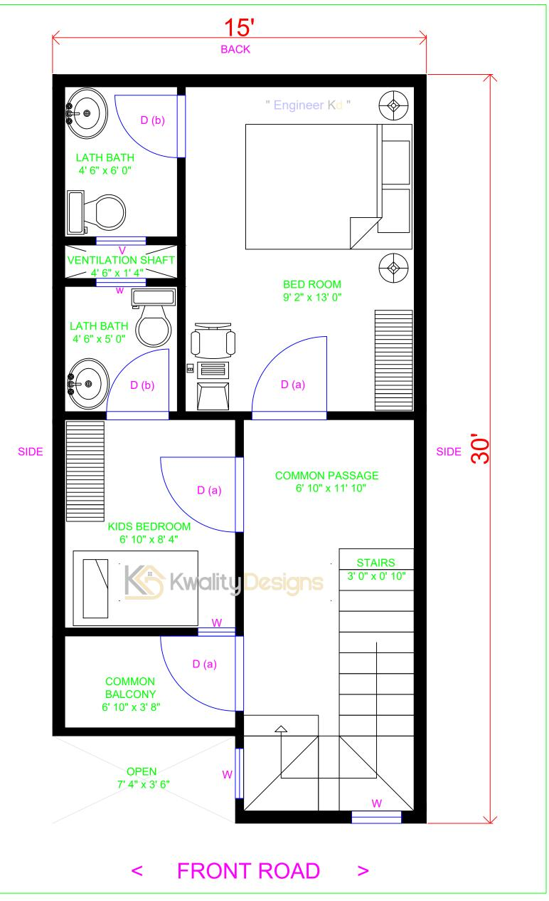
2D PLAN DETAILSOUTER WALL - 6"INNER WALL - 4"COLOUMN - 9" X 9"STAIRS SIZE - 3' X 10"MAIN GATE - 6' WIDEDOOR (D) - 4' WIDEDOOR D (a) - 3' WIDEDOOR D(b) - 2'6" WIDEWINDOW (W)- 2' WIDEVENT (V) - 2' WIDECLIENT NAME: MR. DHARMENDRA SINGHDELHI
